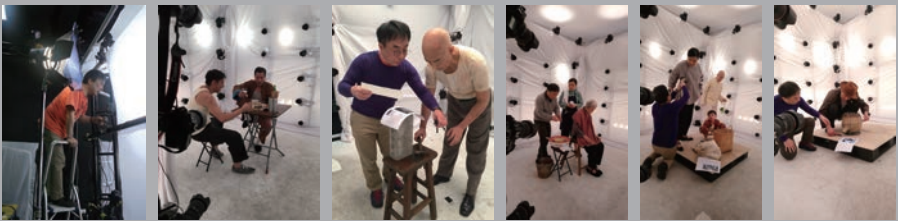
Snap-shots taken during the studio show 70 digital cameras and the lighting equipment that completely surrounds them.
