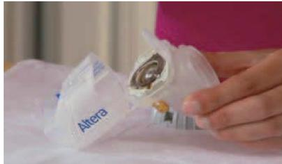
6. Touching ONLY the plastic outer ring of the Aerosol Head, press the 2 flexible plastic tabs on the side of the Aerosol Head and remove it.
