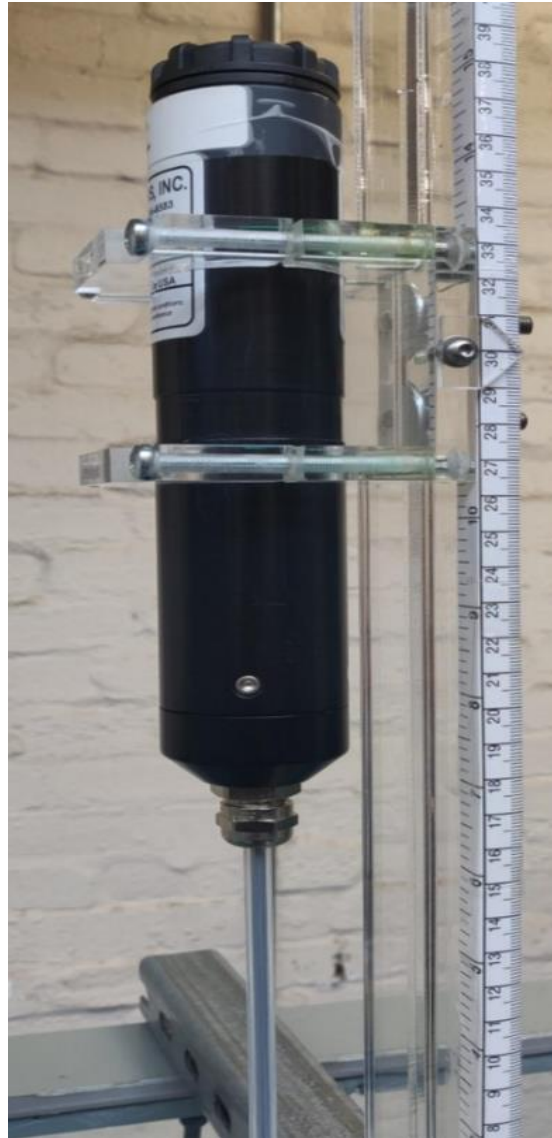
Figure 9 - Wave gauge attached to calibration mechanism.
