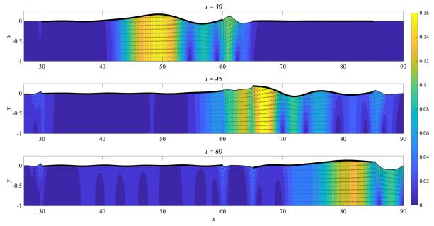
Fig. 2. Vector field and module contours of dimensionless fluid velocity for the interaction of a solitary wave (A = 0.25) with the set of two plates with the same properties  $(L_k = 30, m_k = 0.1, D_k = 5)$  separated by the fluid gap  $(\Delta L = 5)$ .
