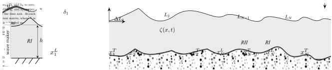
**Fig. 1.** Schematic of the problem of nonlinear wave interaction with N number of deformable plates of arbitrary size and location. The plates may have horizontal motion due to the wave loads. Also shown in this figure are the RI and RII regions referred to in the text.
