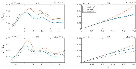
Fig. 4. Variation of the peak of cnoidal wave horizontal force on floating ice sheets with wave length and wave height, for two configurations of a single plate (L=5, m=0.01, D=0.1) and two identical plates of the same properties. In sub-plots (a) and (b), the distance between the two plates is  $\Delta L = L/2$ , and in (c) and (d)  $\Delta L = L$ .
