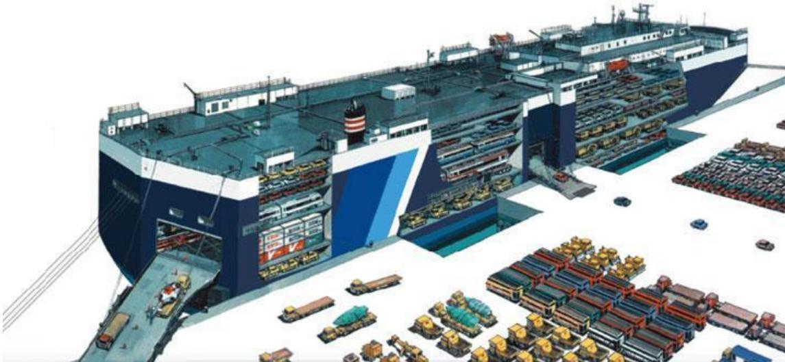
Figure 4.4: External ramp configuration (“RORO Roll On Roll Off”, 2010)
