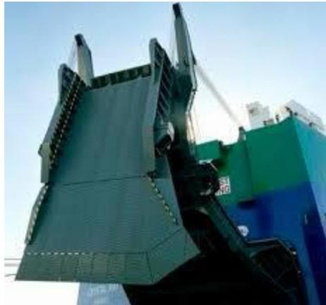
Figure 4.5: Foldable rear ramp (“Quarter Ramp”, 2012)
