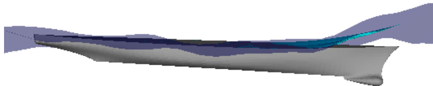
Figure 4. The GW profile at time = 206.70 s for DTMB model 5415 running at 10 knots in Sea State 8, long crested, head seas.
