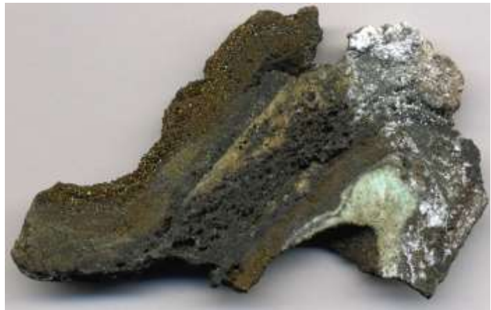
Figure 4: Cross-section of a SMS deposit from a hydrothermal vent. Minerals in this deposit include chalcopyrite (or copper iron sulfide, \text{CuFeS}_2 ), sphalerite (or zinc sulfide, \text{ZnS} ), and anhydrite (or calcium sulfate, \text{CaSO}_4 ) (34).
