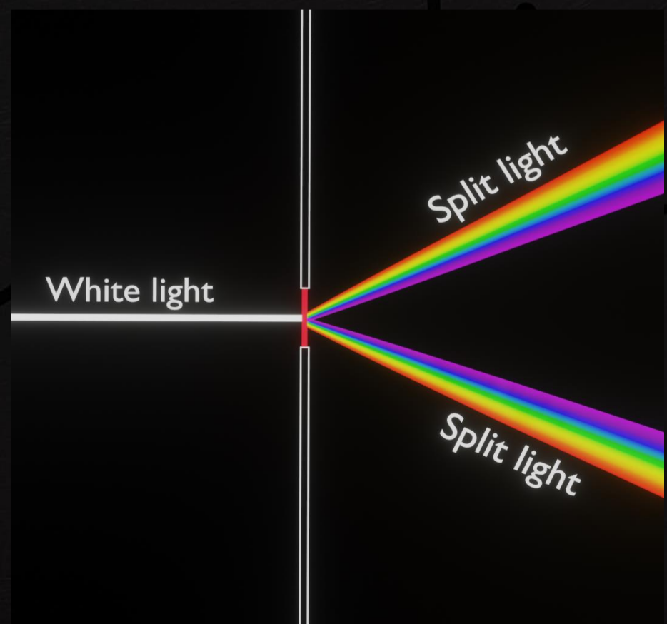
Figure 8 – Shows the effect of splitting light from a source by passing it through a diffraction grating (like how a prism splits light).
