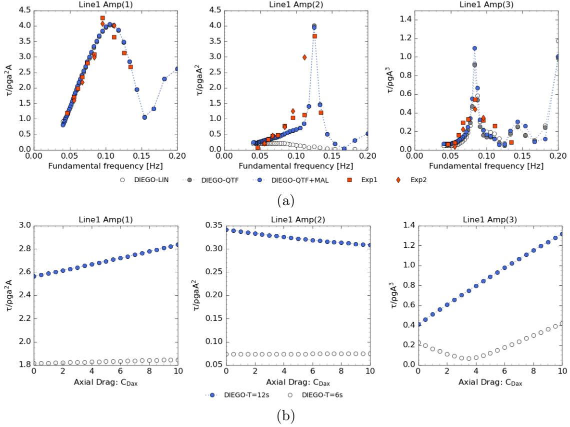
Figure 2: (a) Comparison of EDF-TLP line tension harmonics transfer functions and (b) sensitivity of the springing responses amplitudes to the axial drag coefficient for the upstream Line No1- Potential flow models in regular waves,  $kA=0.10$
