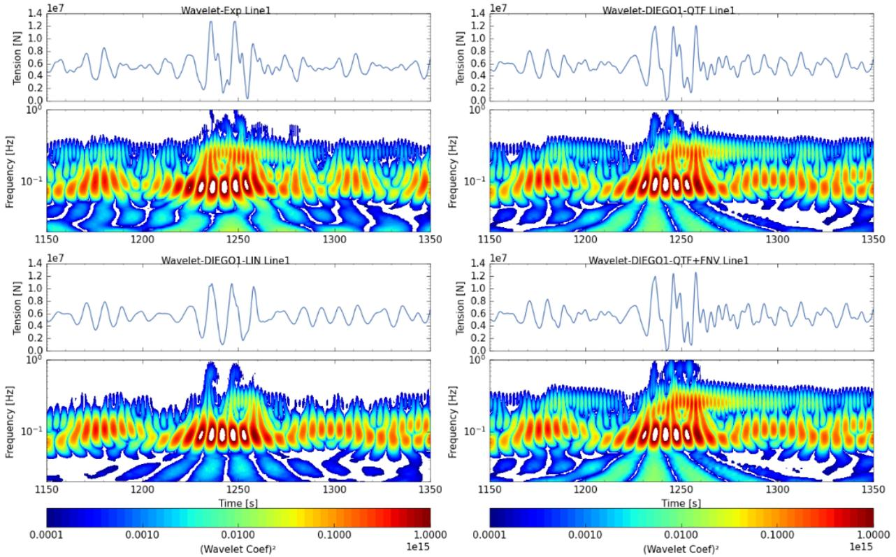
Figure 3: Scalograms of the vertical line tension frequency time-frequency amplitudes of Line No1 for a selected ringing event in irregular wave case EC2a:  $H_s = 9.2$  m,  $T_p = 12$  s and  $\gamma = 3.0$
