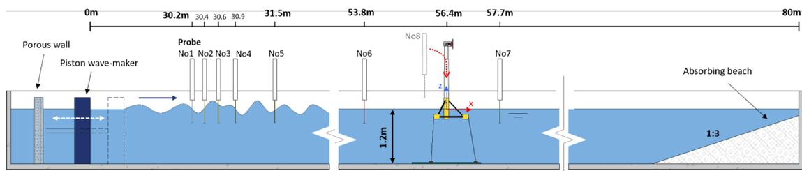
Figure 1: Sketch of the experimental set-up in the wave flume
