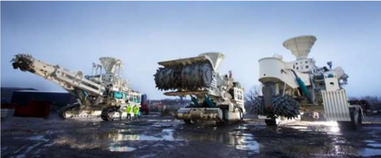
Figure 11: Machinery owned by Deep Sea Mining Finance Ltd (“DSMF”; previously Nautilus Minerals Company) for exploitation of seabed minerals. From left to right: ‘Collection Machine’, ‘Bulk Cutter’, and ‘Auxiliary Cutter’ (94). For size, note the workers for reference in front of the Collection Machine on the left.
